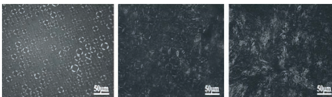
Fig. 6: Liquid crystalline structures under the microscope and polarized light: (1) liquid-crystalline emulsion in globular structure (so-called „Maltese crosses“), (2) the same emulsion directly after application (globular structures are still visible but already lamellar structures can be detected), (3) – same emulsion 10 min after application changed to lamellar structures
